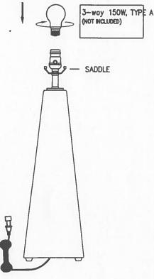
CAUTION: IN ACCORDANCE WITH THE UL REGULATION, THE SHADE SHOULD BE OPEN TOP & OPEN BOTTOM AND "CD" IS BIGGER THAN OR EQUALS TO  $4\frac{1}{2}$ ", "R" IS NOT SMALLER THAN  $4\frac{3}{4}$ " OR MAY CAUSE FIRE. "H" IS  $3\frac{1}{4}$ ".
